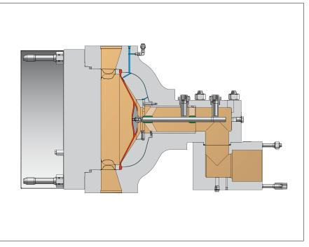
High-pressure diaphragm housing minimizes stress in clamping rim area.
