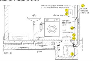
In case of installation beneath the backpressure level the pressure tube must be taken in a loop over the local backup level acc. to EN 12056. Besides, it must be secured with a EN 12050-4-proofed swing-type check valve. Additionally we recommend an alarm system.
