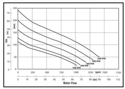
The PrimeRite™ pump performance is based on clean water at sea level, with 10' suction lift. With the standard diesel engine, the CT004 will perform up to 1800 RPM.
