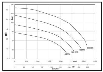
The PrimeRite™ pump performance is based on clean water at sea level, with 10' suction lift. With the standard diesel engine, the CT008 will perform up to 2000 RPM.
