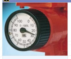
Flow rate adjustment is smooth and linear, and can be made whether the pump is running or stationary.
