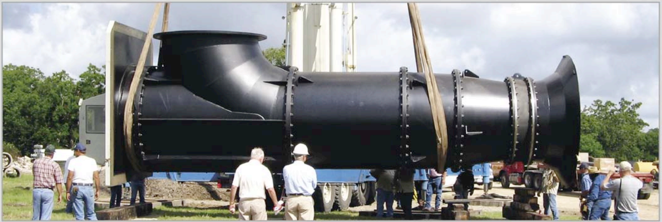
96-in., 260,000-gpm Axial Flow Pump for Velasco Drainage District in Texas.
