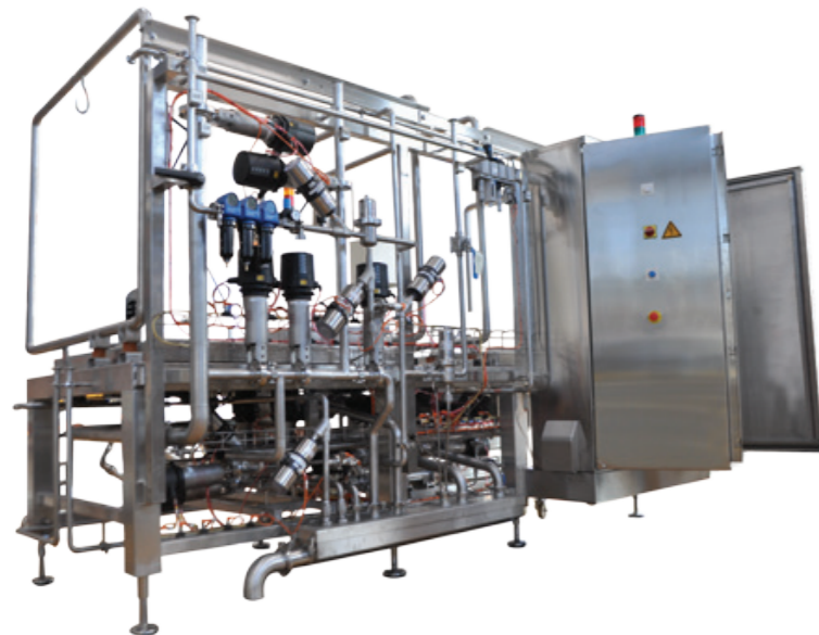
Dosyfruit™ Compact Multi ingredients, automatic valves, minimum fruit losses between productions and containers below the station
