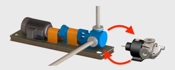
No piping changes: Port size and locations match No driver changes: Nominal input power matches No coupling changes: Drive shaft size matches No flow rate changes: Nominal flow rate matches
