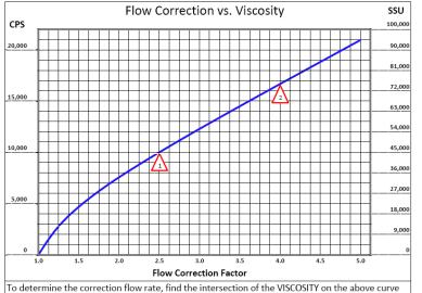
and read the FLOW CORRECTION FACTOR. Multiply this factor by the desired flow of the pump and use this new flow rate to select a pump from the performance curves.
