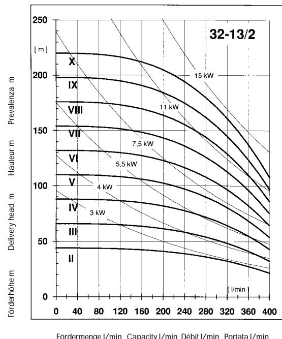
Fördermenge l/min Capacity l/min Débit l/min Portata l/min
