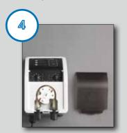
Continue to feed tube until it locates into housing slot.
