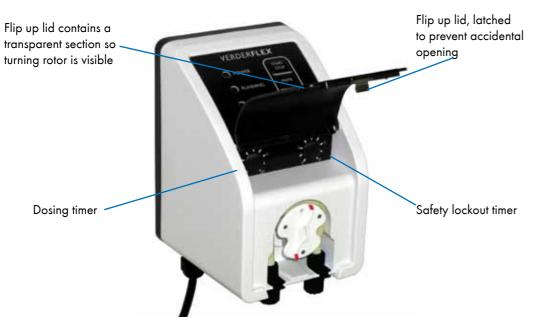
Both timers have removable tamper evident plugs with screwdriver slot adjustment, preventing unauthorised adjustment.
