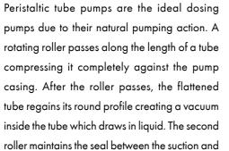
discharge sides, trapping the medium and pushing it out on the delivery side of the pump.
