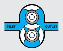
**For High Viscosity Fluids,** the large fluid cavities of the rotors... plus the large, easy entry anti-cavitation ports... allow efficient pumping of high viscosity fluids, slurries or even liquids with large chunks or particles.
