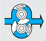
For Non-Lubricating and Abrasive Fluids, the unique Waukesha Cherry-Burrell design has no bearings in the fluid being pumped, no sliding or rolling contact and no rotor-to-rotor contact. This produces MAXIMUM SERVICE LIFE even under severe operating conditions.
