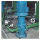
Pump: KF 20 bis KF 550. Medium: Polyol, isocyanate. Delivery rate: 282 l/min. Speed: 750 min<sup>-1</sup>. Pressure: 10 bar. Temperature: Ambient. Viscosity: Polyol to 5.000 mm²/s, isocyanate to 1.500 mm²/s. Seal: Magnetic coupling.
