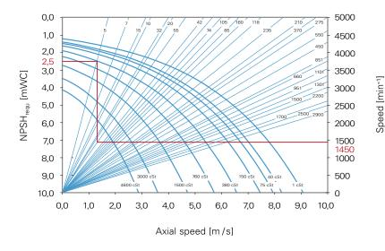
The NPSH-value (Net Positive Suction Head) indicates by how much the total pressure head at the pump inlet has to exceed the vapor pressure head pd of the liquid to avoid cavitation. The available absolute pressure head is reduced by the suction head  $\Delta h_s$ , the pipe loss  $\Delta h_v$  and a safety margin of 2 mWC.
