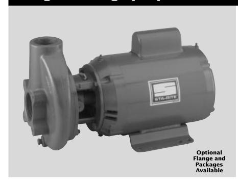
These Sta-Rite pumps are compact and lightweight, but rugged. Choose from 3 or 5 HP high head and medium head models. For lower pressures and maximum capacity, medium head models offer heads to 75 feet and capacities to 220 GPM. Where higher pressures are desired, the high head model offers heads to 102 feet and capacities to 260 GPM.
